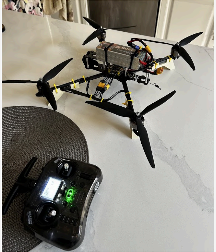
Figure 0.1. 10" drone with custom raised legs
